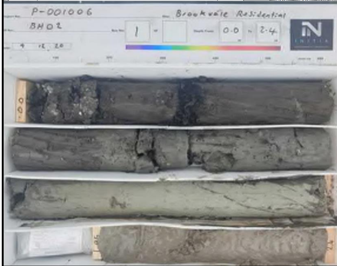
Figure 6. Upper 2.0 m detailed bore log data and photo for the for Bh2.
